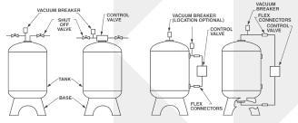
NOTE: Flexible connectors must be installed between hard piping and tank openings. These pressure vessels are treated for an internal negative pressure of 5y HG (17 Pa) vacuum below atmospheric. If negative pressure could ever exceed 5y Hg (17 Pa), an adequate vacuum breaker must also be properly installed. Failure to install flex connection properly, or improper installation of a vacuum breaker when required, may void the warranty.
